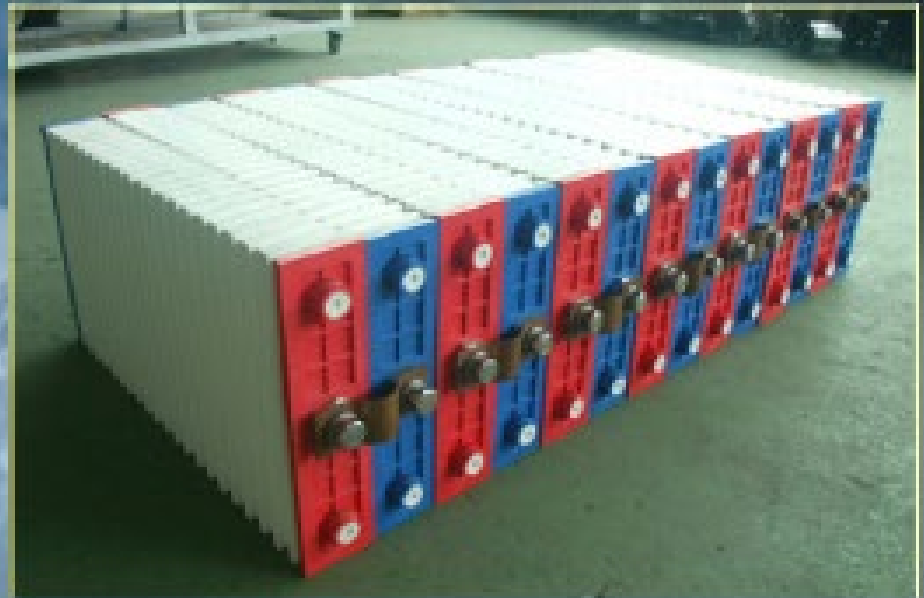
(b1) 48V 500Ah battery pack with out of phase electrodes
